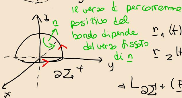
$$\begin{aligned} r_1(t) &= (0, R\cos t, R\sin t), \quad t \in [0, \pi] \\ r_2(t) &= (R \cos t, R \sin t, 0), \quad t \in [-\frac{\pi}{2}, \frac{\pi}{2}] \\ \Rightarrow L_{\partial\Sigma^+}(F) &= L_{\gamma_1}(F) + L_{\gamma_2}(F). \end{aligned}$$
