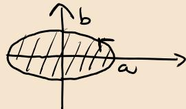
$$\begin{aligned} r(t) &= (a \cos t, b \sin t), \quad t \in [0, 2\pi] \\ r'(t) &= (-a \sin t, b \cos t) \end{aligned}$$
