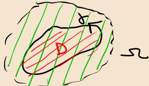
Poiché:  $L_{\partial D^+}(\underline{F}) = \iint_D (\text{rot } \underline{F} \cdot \underline{k}) dx dy$
